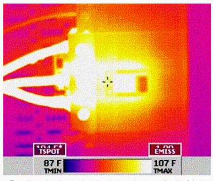
Thermal image that shows overheated conductors and contacts on line side of circuit breaker (photo credit: irinfo.org)
