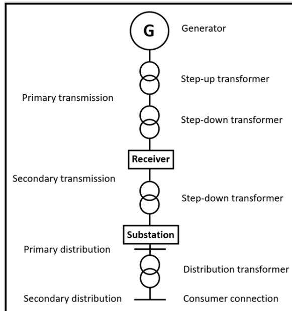
Figure 10: A simple diagram of the national transmission and distribution network.
