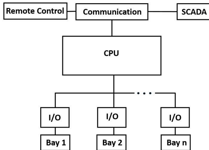
Figure 1: Conceptual CPC system architecture.
