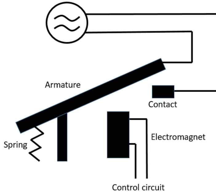
Figure 11: A schematic picture of a classical electromechanical relay circuit.
