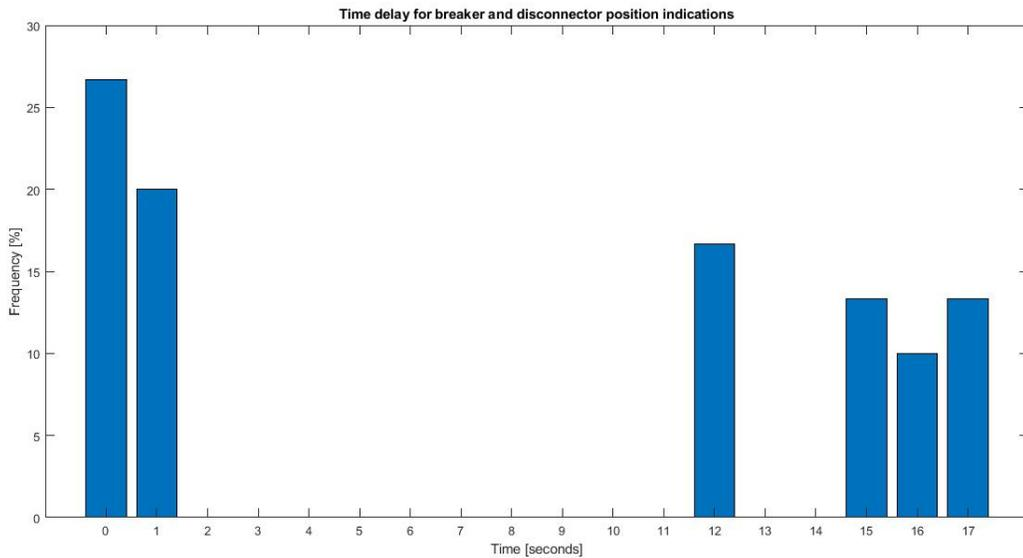
Figure 46: Frequency of each time delay for messages concerning switchgear position indications.
