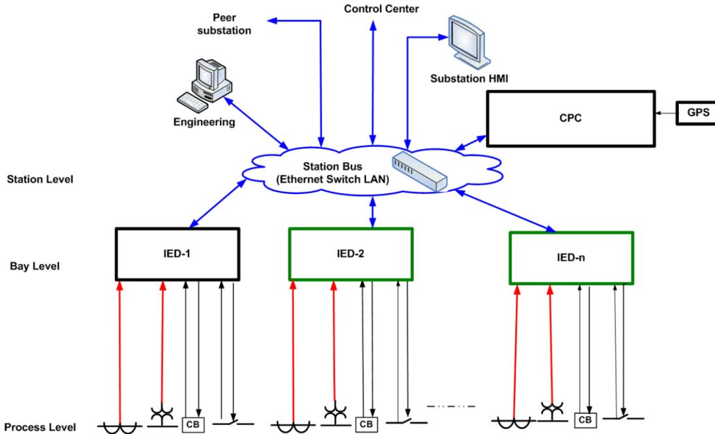
Figure 2: CPC system architecture with the central computer only performing backup and redundancy duties [1].
