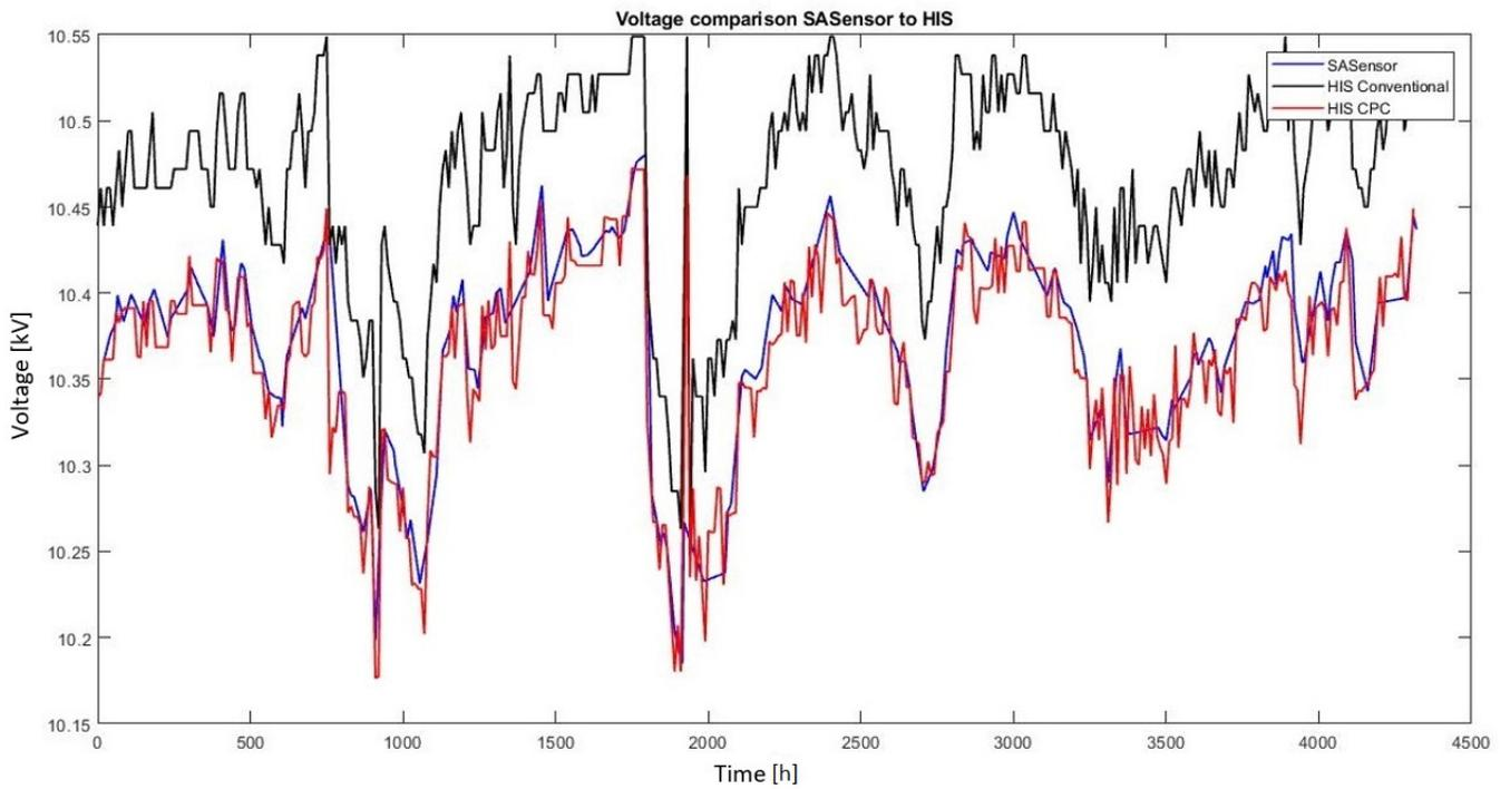
Figure 40: Voltage signals from HIS and the centralized system logs over three days
