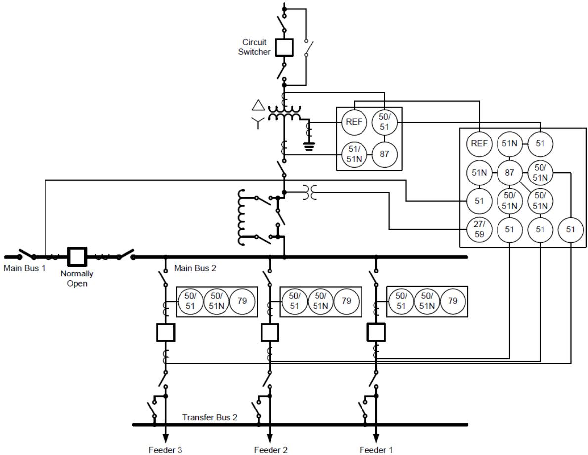
Figure 14: The protection scheme developed by MCEC.[12]
