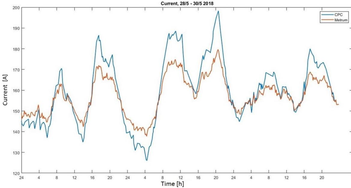
Figure 43: Current signals from HIS and the centralized system logs over three days.
