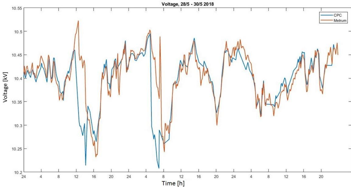
Figure 42: Voltage signals from HIS and the centralized system logs over three days
