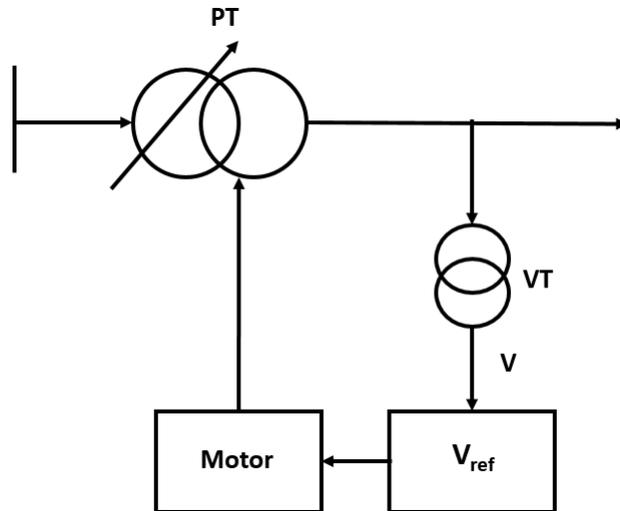
Figure 16: A schematic of a tap changing feedback loop.[12]
