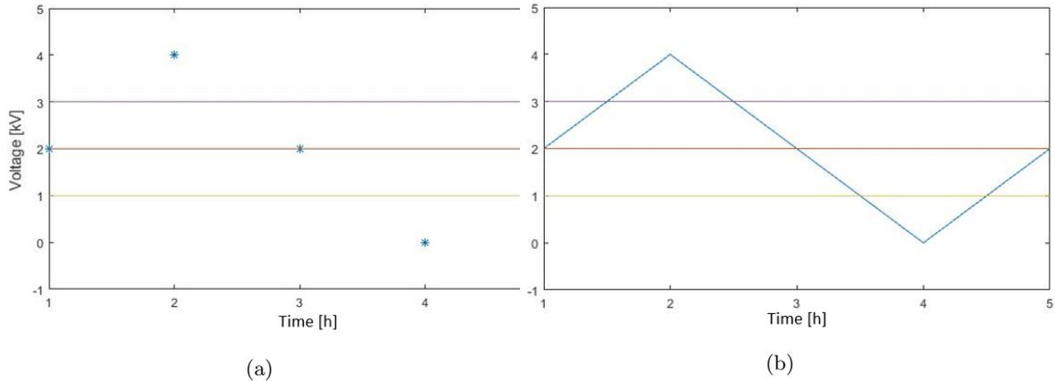
Figure 34: A representation of how the regulation time is calculated. a) A plot of the vector with the elements represented as points on a graph. b) Linear interpolations between the elements. The regulation time is the time from when the line crosses a limit until it returns.
