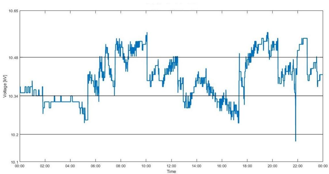
Figure 33: An example of voltage data read from HIS, taken from the substation as one second averages during the first of March, 2017.
