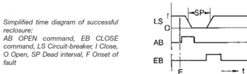
Figure 12: A diagram of an autoreclosing event.[7]
