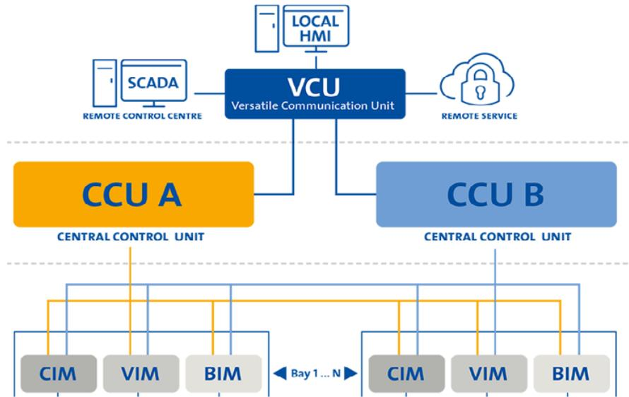
Figure 6: The system architecture of SASensor. The BIM, CIM and VIM modules only measure data and perform no data analysis, all advanced processing and communication is performed by the control and communication unit, respectively [14].
