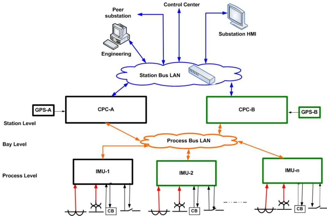
Figure 3: CPC system architecture with the central computer performing all protection and control with no IED autonomy [1].
