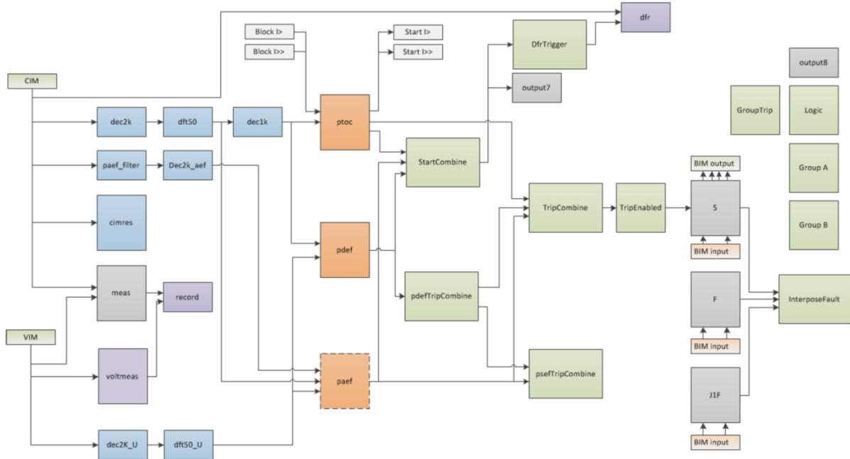
Figure 23: Function block overview of the class for the incoming overhead line.
