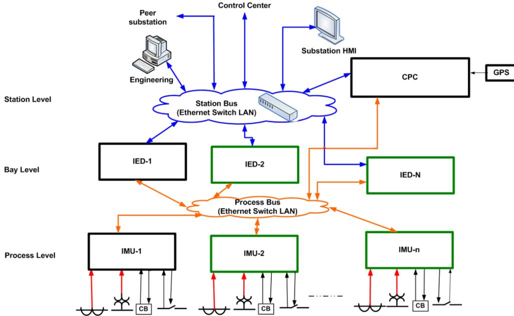
Figure 4: CPC system architecture with both the central computer and IEDs performing protection and control. The duties of the respective systems can be distributed after user preferences [1].
