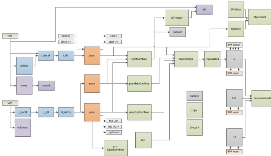
Figure 26: Function block overview of the class for the incoming bay.
