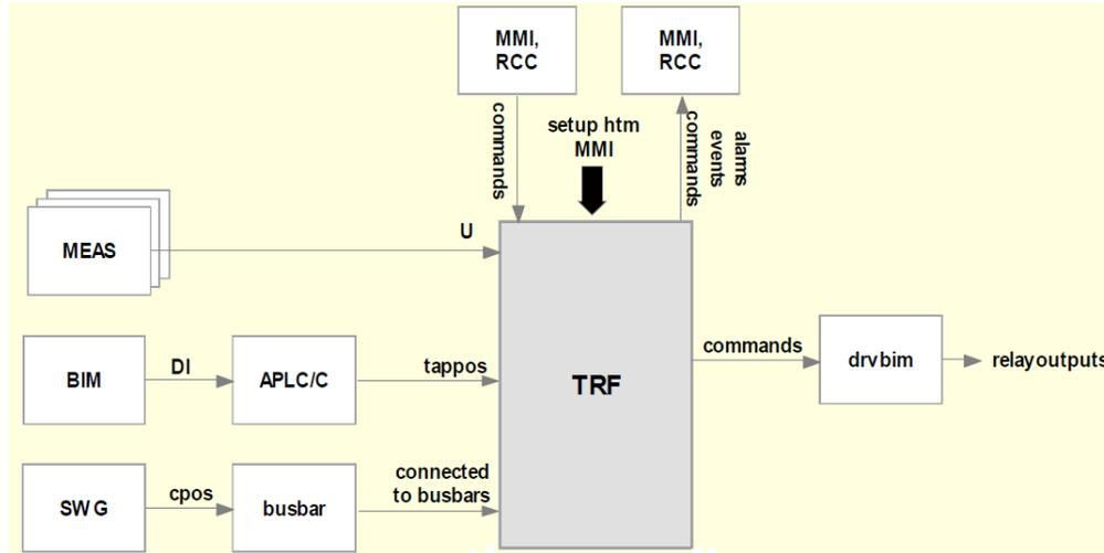
Figure 29: Functional overview of the voltage regulation function in SASensor.[30]
