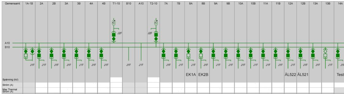
Figure 22: The interface representation of the 10 kV side of the station.
