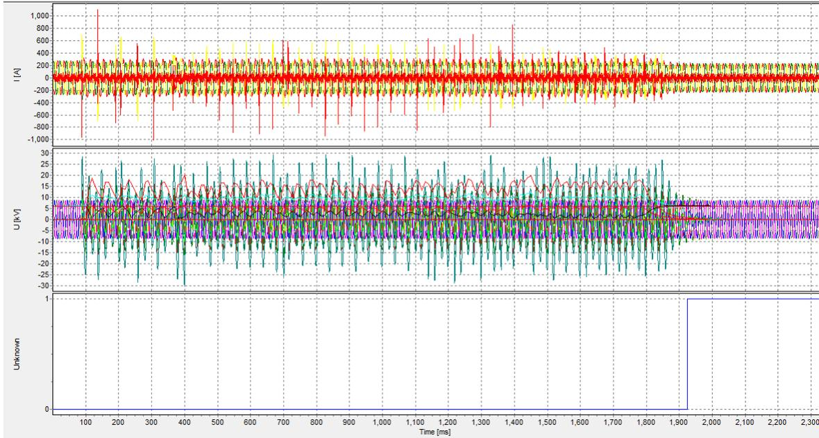
Figure 47: The active signals recorded by the DFR in the earth fault.
