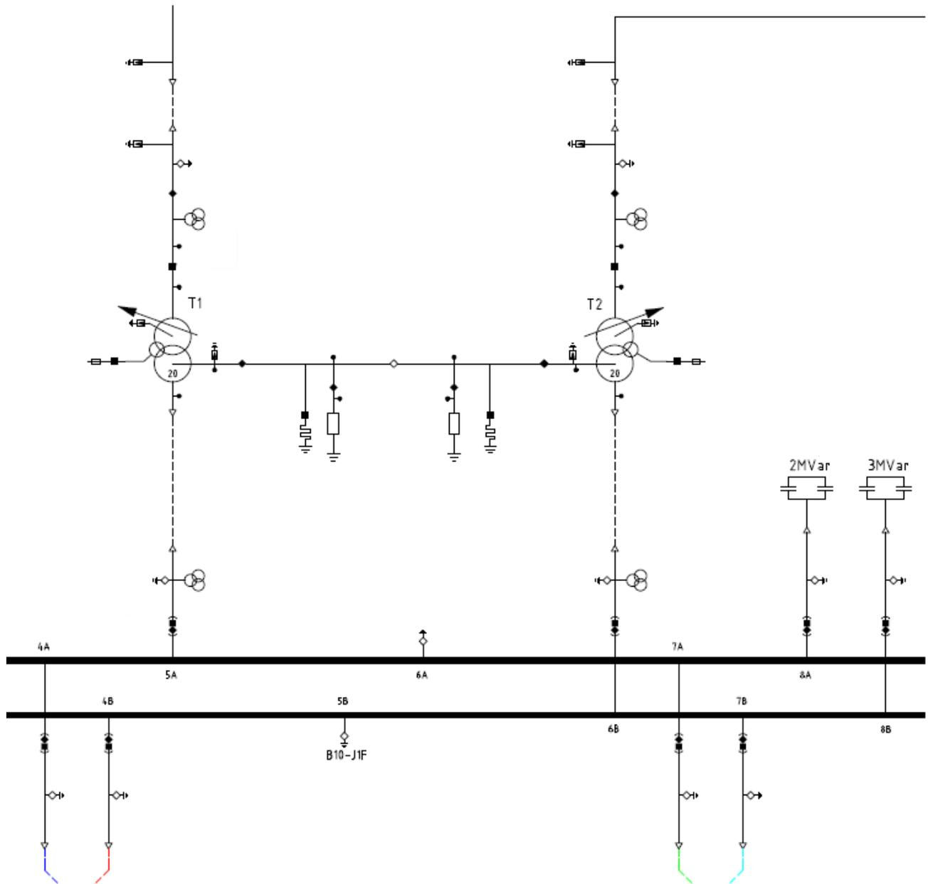
Figure 20: single line diagram of the substation.
