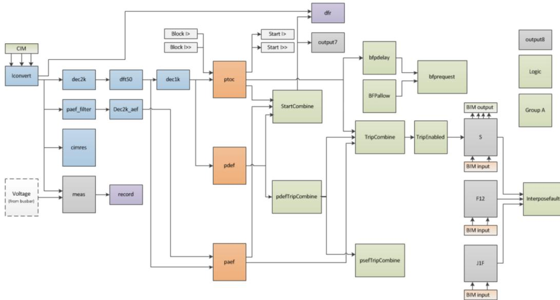
Figure 27: Function block overview of the class for the outgoing bay.
