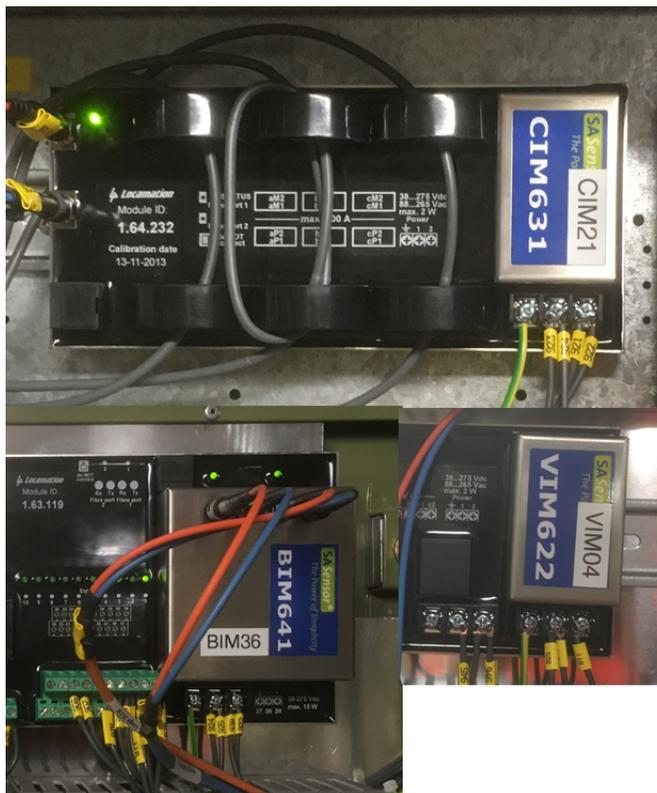
Figure 9: The three interface modules: CIM, VIM and BIM.
