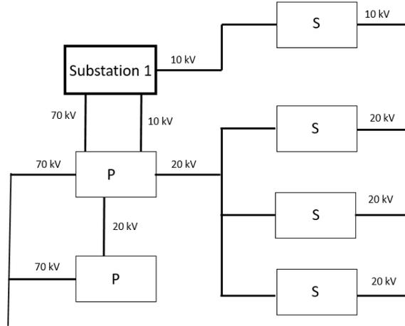
Figure 18: Schematic of the surrounding grid with all voltage levels. The substation in the study is named "Substation 1". The primary substations (P) transform the electricity from high ( $>50$  kV) to medium voltage (between 50 and 1 kV) and the secondary (S) from medium to low voltage ( $<1$  kV).
