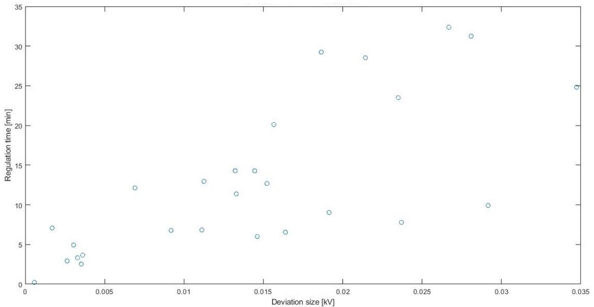
Figure 38: Time delay characteristic of the voltage regulation.
