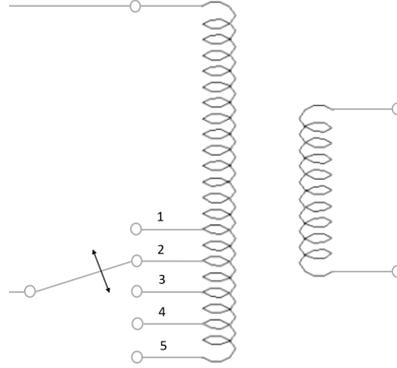
Figure 15: A schematic of a tap changing device.
