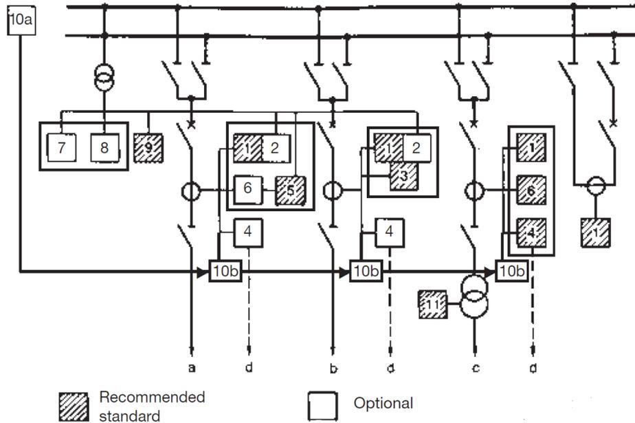
Figure 13: A standard ABB protection scheme for two busbars, one transmission line, one cable and one transformer.
