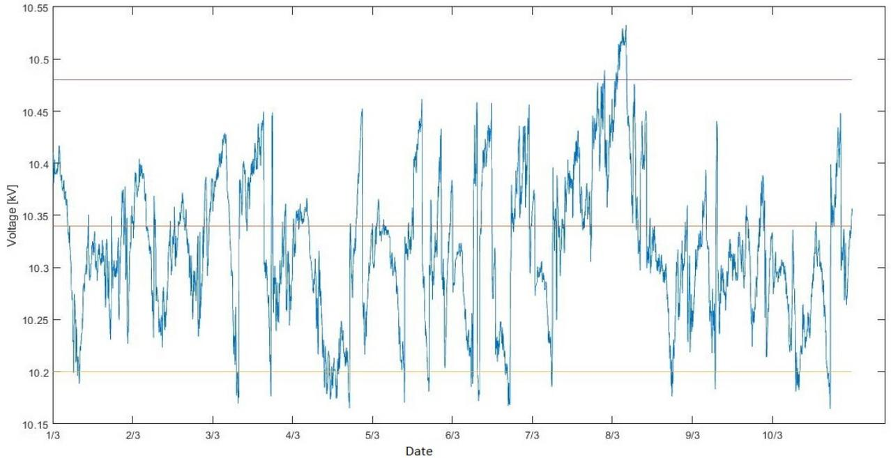
Figure 37: Voltage data from 1/3 to 10/3 2017. The time resolution is five minutes. The lines indicate the set voltage and the lower and upper voltage limits.
