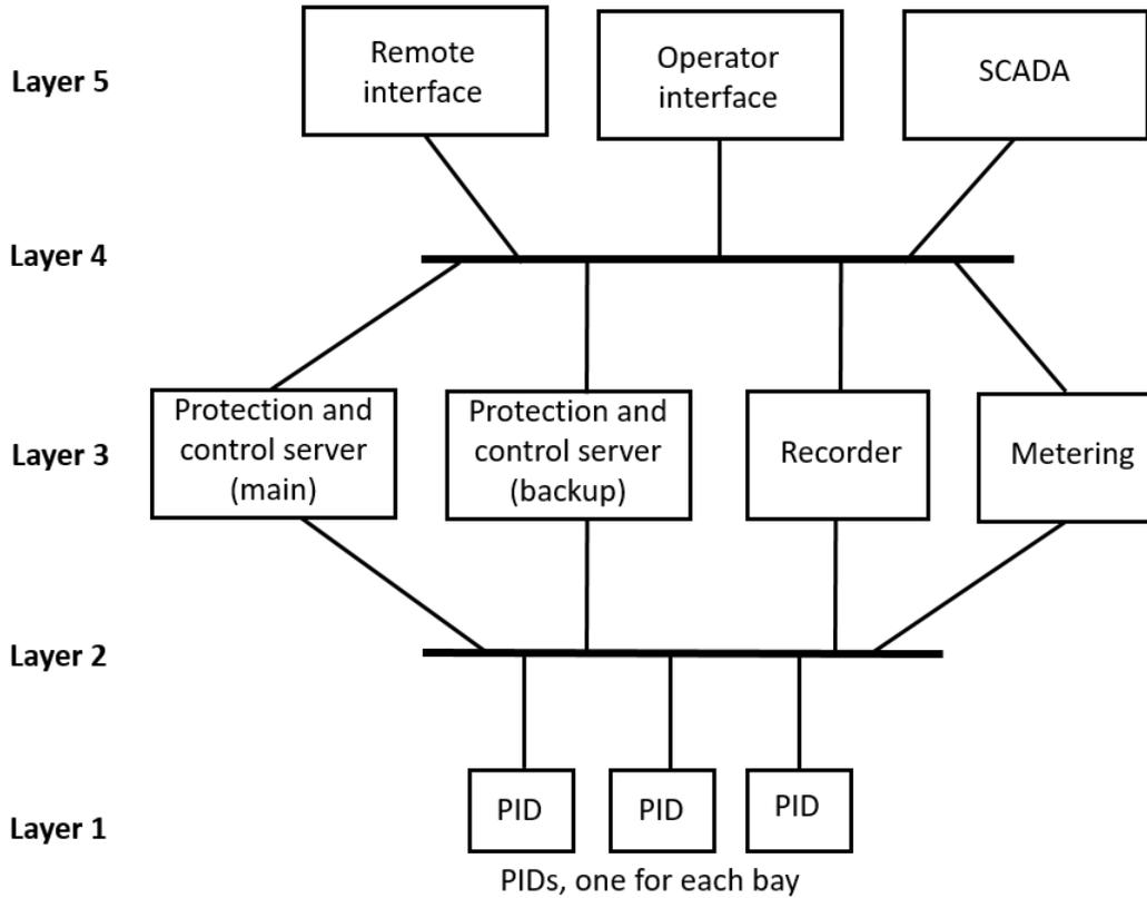
Figure 5: The system architecture of iSASarch. It is made up of five layers, each with well defined, exclusive duties [1].
