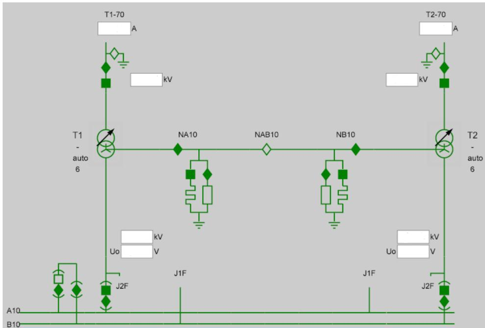
Figure 21: The interface representation of the 70 kV side of the station.
