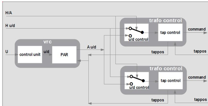
Figure 30: Functional overview of the TRF function block in SASensor.[30]
