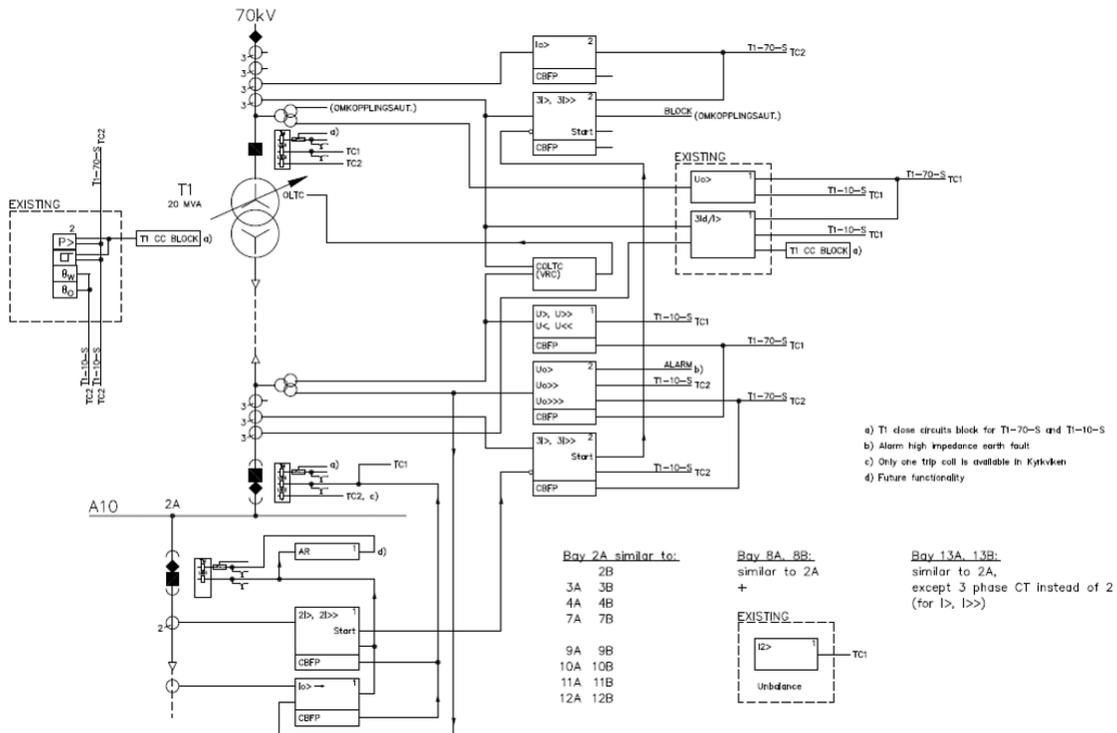
Figure 28: Overview of the conventional relay protection system [23].
