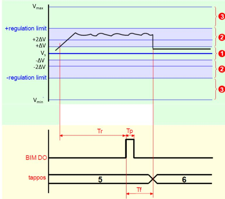
Figure 31: Time/Voltage diagram showing the voltage regulation function's response to a voltage deviation.[30]
