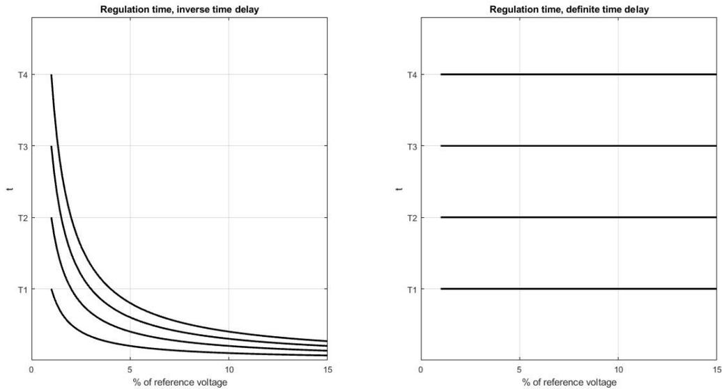
Figure 17: Inverse and definite time delay. For inverse delay, the delay time shortens with higher regulation error. For definite delay, the delay time is constant regardless of regulation error.
