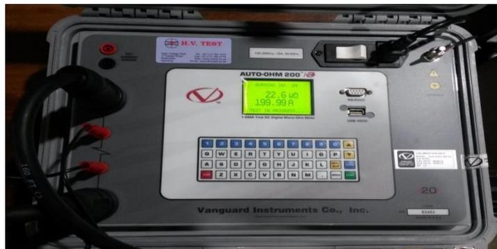
**Figure 2-11: Vanguard Auto-Ohm 200 S3 true dc micro-ohmmeter**
