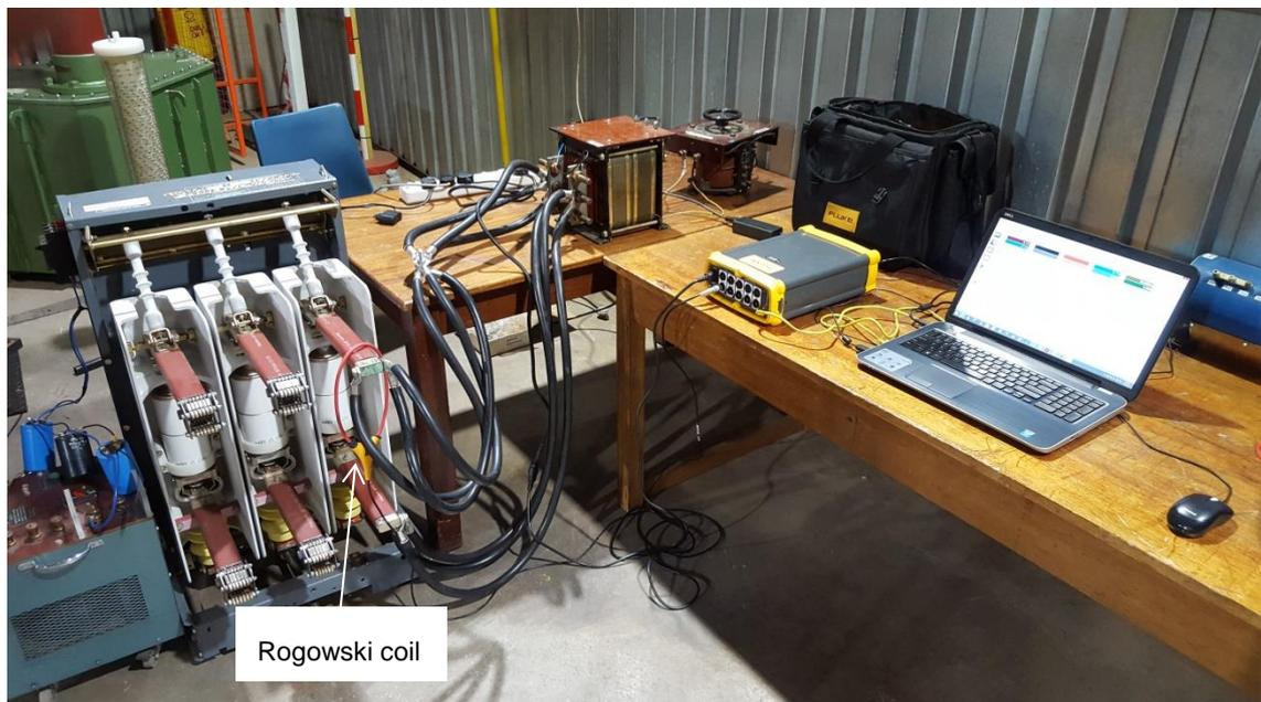
**Figure 4-15: Measuring the chopping current of vacuum interrupters rated at 1250A**
