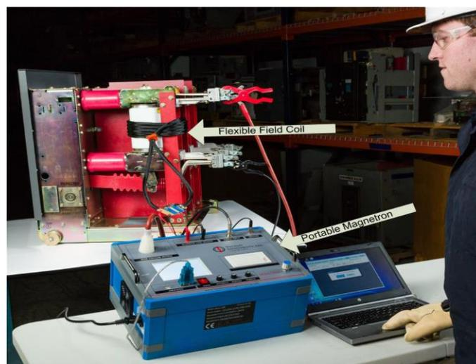
Figure 2-14: Vacuum interrupter pressure measurement with portable magnetron [28]
